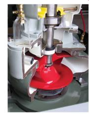
Guide bearing (self-metering design prevents overgreasing)
